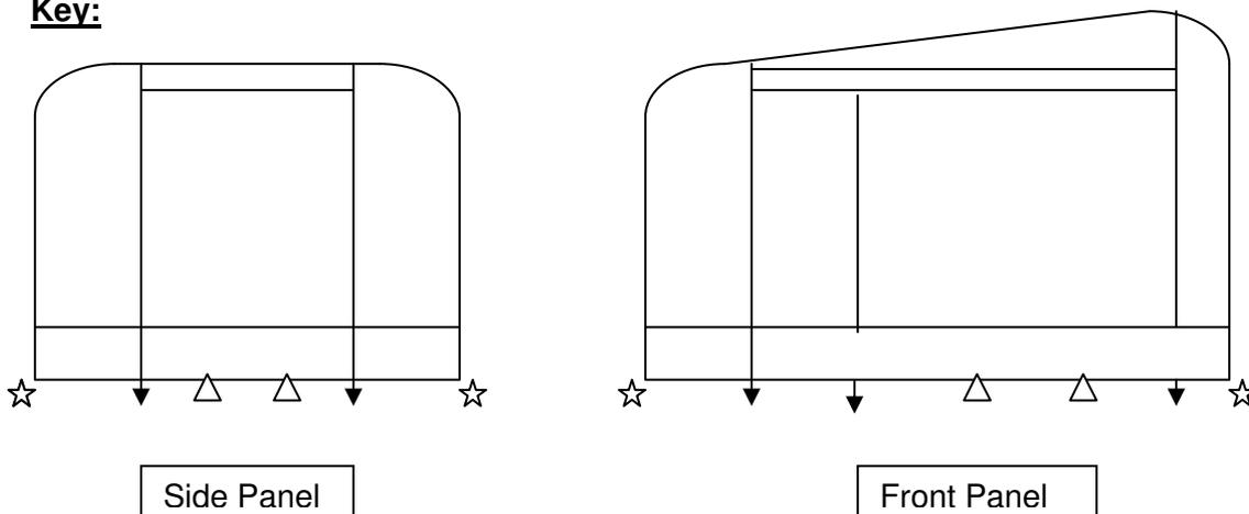
The “flexi-peg” clips ( △ ) are fitted by simply sliding them onto the piping fitment from one end (a fixed clip is fitted at each end ☆ ) and positioning them where desired. When fitting the clips you should ensure that they are fitted **no more than 75 cms apart** and, in particular ( ↓ ), one must be positioned at the bottom of all vertical seams (as shown).
